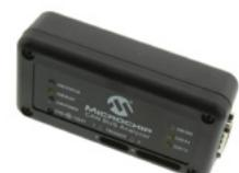
intended to be a simple to use low cost CAN bus monitor which can be used to develop and debug a high speed CAN network.
